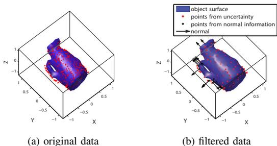
Fig. 5: An example to illustrate the performance of the GP-based filter. **Left:** 500 datapoints are randomly sampled from the point cloud of a jug, obtained from a 3D scanner. The surface is reconstructed with the method in [12]. **Right:** With the filter, only 120 datapoints are selected, either according to their prediction uncertainty (red dot) or from their normal information (black dot and arrow).
