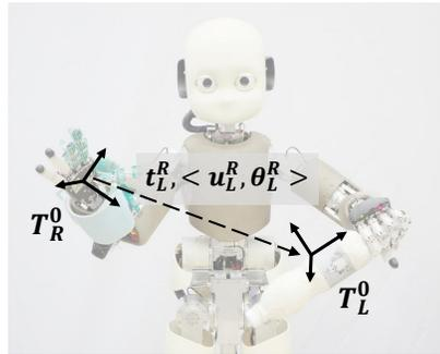
Fig. 2: Schematic of the bimanual constraint. The frames  $\mathcal{T}_0^L$  and  $\mathcal{T}_0^R$  of the interest points should coincide to satisfy the bimanual constraint. The frame  $\mathcal{T}_0^L$  changes depending on where the object should be scanned and the estimation of the object’s diameter.
