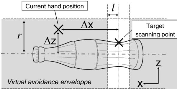
Fig. 3: Scheme of an object and its collision avoidance virtual envelope. A lateral safety zone is delimited by the parameter  $l$ , in which the exploring hand can enter. The diameter of the virtual envelope is defined by  $r$ .
