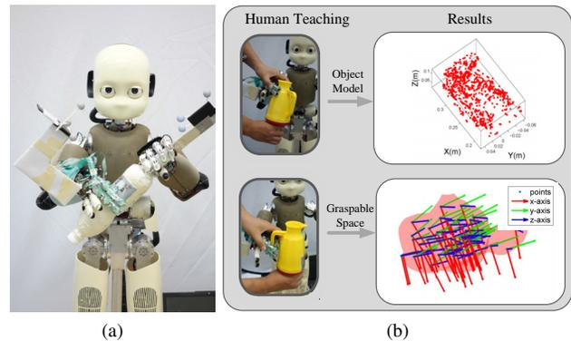
Fig. 1: **Left:** The iCub humanoid robot is exploring an object with its two hands. **Right:** The robot is taught the shape of the object by a human teacher passively guiding the robot's hand along the object, emphasizing the object's part that can be grasped, e.g. the handle on the jar. The object model is stored as a point cloud and the graspable part is modeled using GMM (Gaussian Mixture Model).
