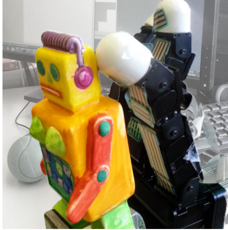
Figure 4.22: Exp 4: Failure with the statuette: the part in contact (the tip of the fingertip) is not sensorized.
