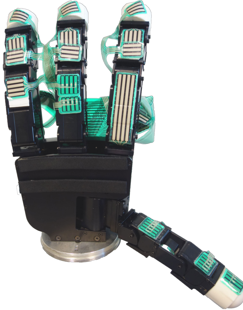
Figure 4.19: The AllegroHand with fingers covered with Tekscan tactile sensors. Each patch is a matrix of 4 \times 3 or 4 \times 4 taxels ( 4 \times 15 for the base of the index finger). The Tekscan sensors are designed for human hands, so the mapping from tactile patch to fingers is customly adapted to the AllegroHand .
