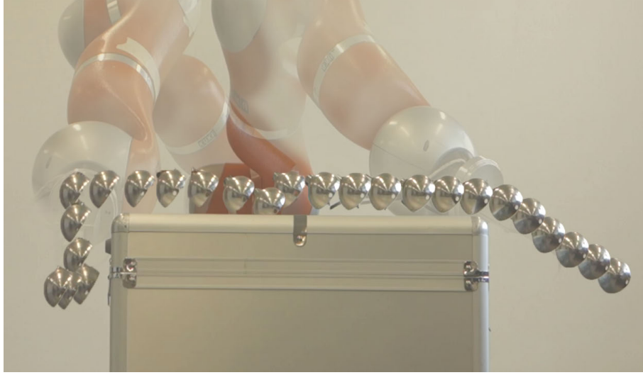
Figure 5.19: Exp 2a real robot: Trajectory of the end-effector during the task with one large obstacle. The end-effector collides on the side of the object and another time on the top.
