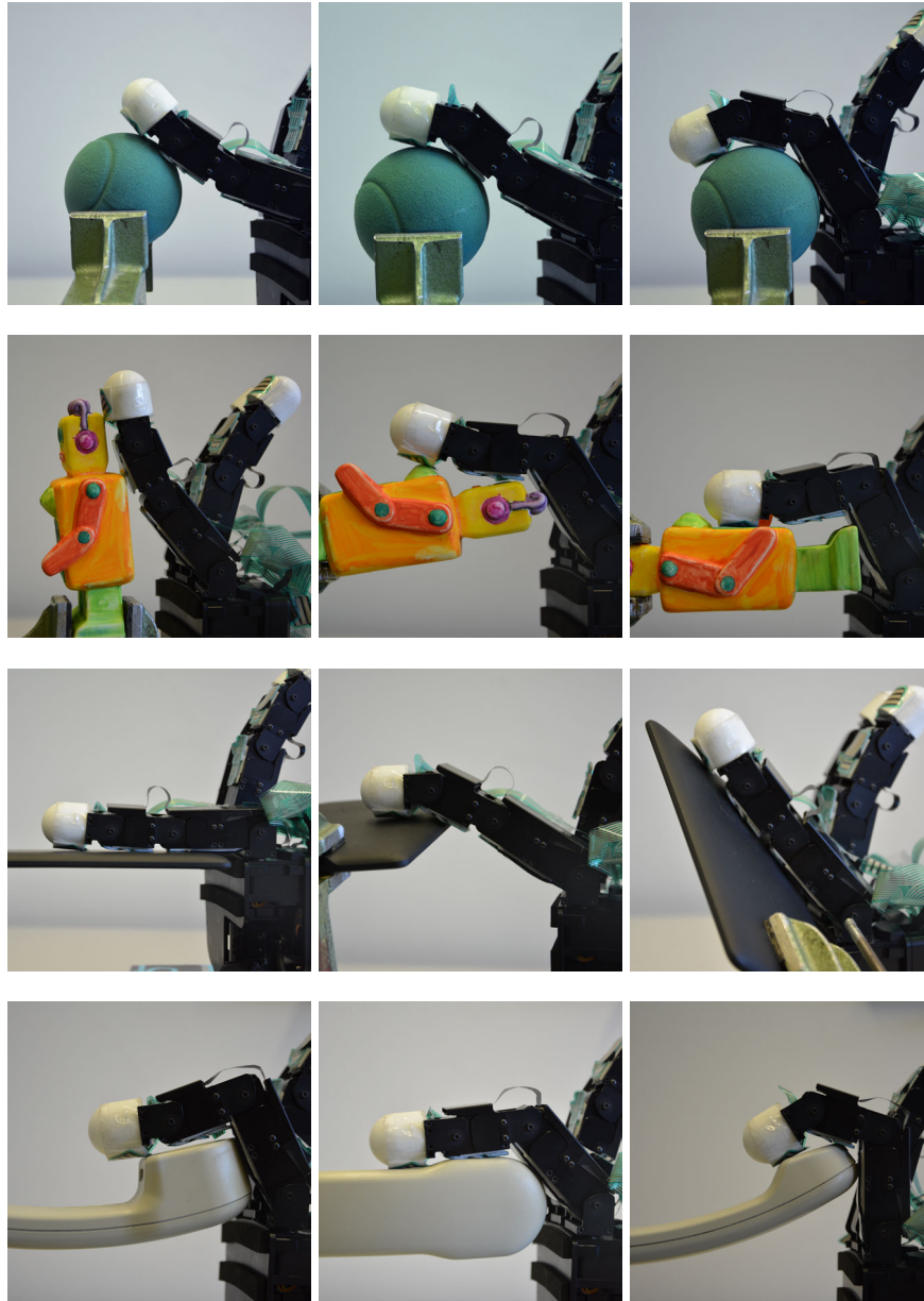
Figure 4.21: Exp 4: The 3 poses/orientations for each object (in order a,b,c), with the corresponding "optimal" contact posture obtained by active compliance with the object. The initial finger configuration is palm flat open upwards, see Figure 4.19.
